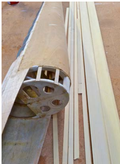
Clockwise from left: Kaihikatea being planed to the required thickness. The ply-covered fuselage dorsal section and Kaihikatea strip All moving tailplane and Petrel 3 view.
